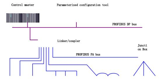
Figure 4.1 PROFIBUS PA network topology
