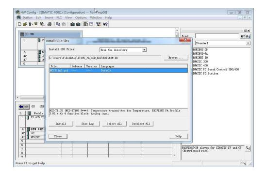
Figure 4.5 Installing the GSD files
