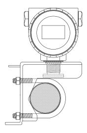
Figure 2.4 curved bracket tube installation 2
