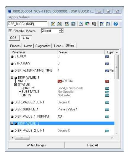
Figure 3.6 Parameter configuration for display block
