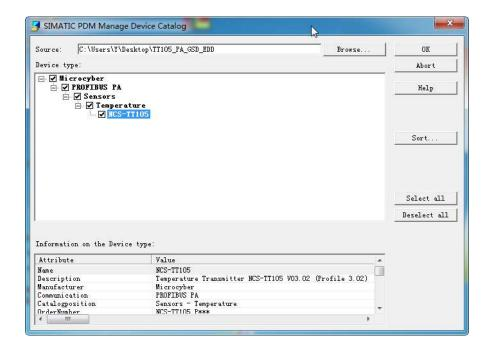
Figure 4.8 Selecting a Device Type
