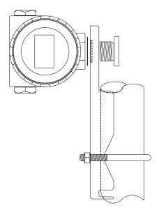
Figure 2.1 Flat bracket tube installation
