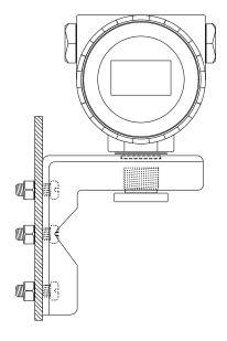
Figure 2.2 Curved bracket plate installation
