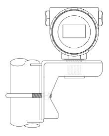
Figure 2.3 curved bracket tube installation 1
