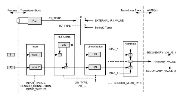
Figure 4.3 transducer block structure
