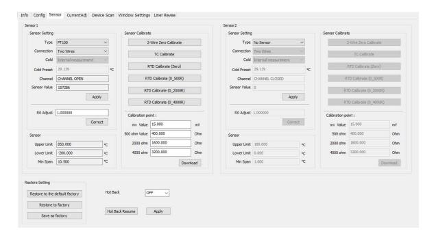
Figure 5.5 Sensor Configuration
