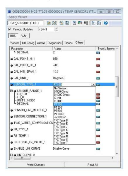
Figure 3.3 Sensor type configuration
