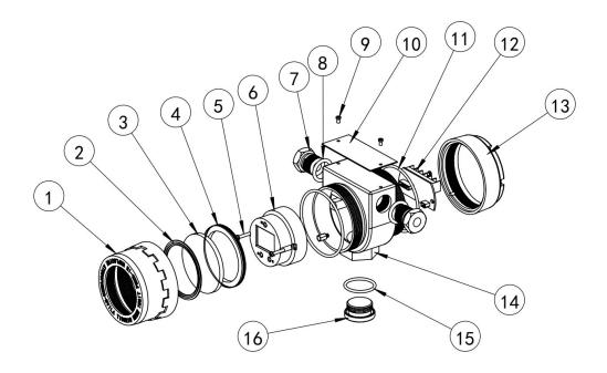
Figure 1.2 The general assembly drawing
