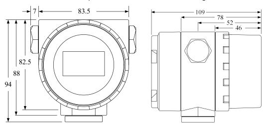
Figure 1.1 Dimensions of temperature transmitter (unit: mm)
