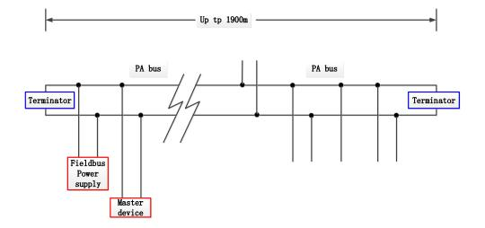
Figure 4.2 PROFIBUS PA bus connection
