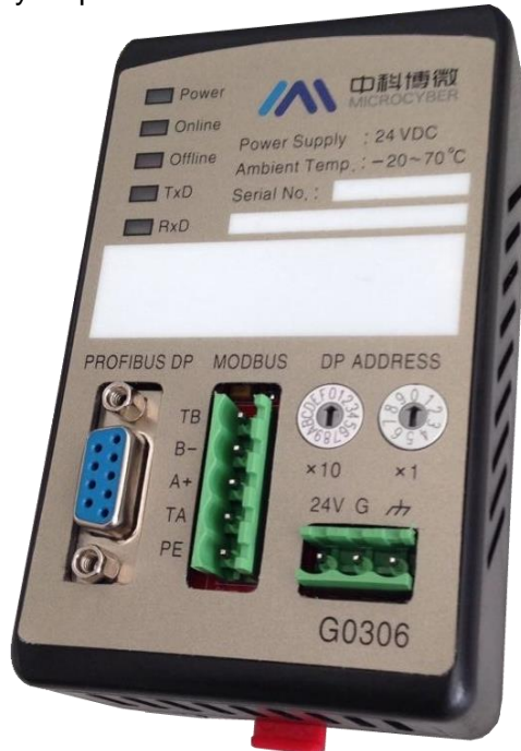
Figure 1 G0306 Modbus to DP Gateway
