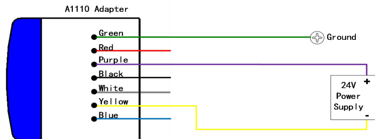
Figure 3-2 Wiring Diagram of A1110 as Repeater
